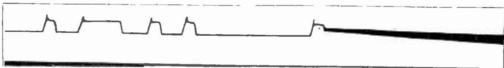
FIG. 12.—THE SIPHON PEN, ON THE RIGHT, TRACING OUT IN MORSE ALPHABET. THE FIRST WORD—"LE"—OF COMMANDANT FERRIÉ'S MESSAGE
